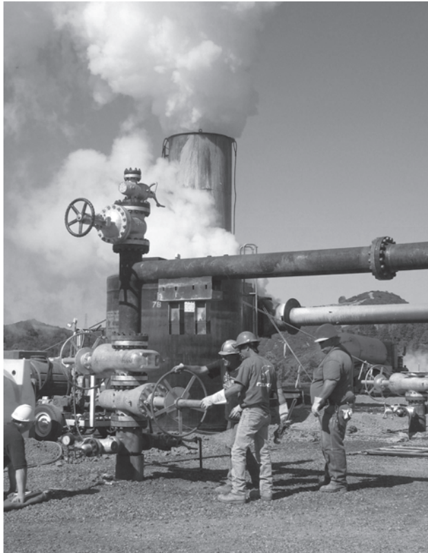
Opening the well head valves on West Coleman 4-6 during flow test and gathering pressure build-up data.
